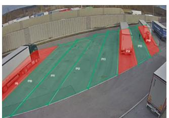
Real-time parking data collection by using an entry-exit-counting system or by single parking space detection. Similarly to traffic surveys, an entry-exit-counting system counts entries and exits to determine the current parking utilization through the difference between them. As an alternative, the utilization can be determined by recording the individual parking spaces. The image material is evaluated and vacant and occupied parking spaces are identified.
